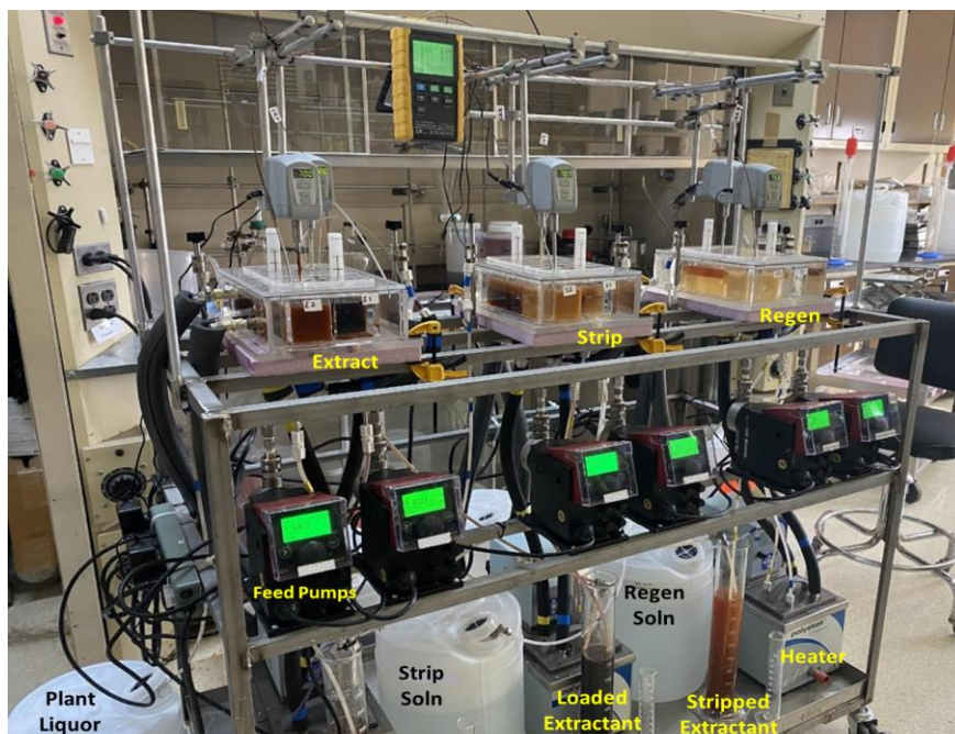
Figure 14. Photograph of the laboratory scale SX circuit in a cart (total flow = 40 mL/min).
